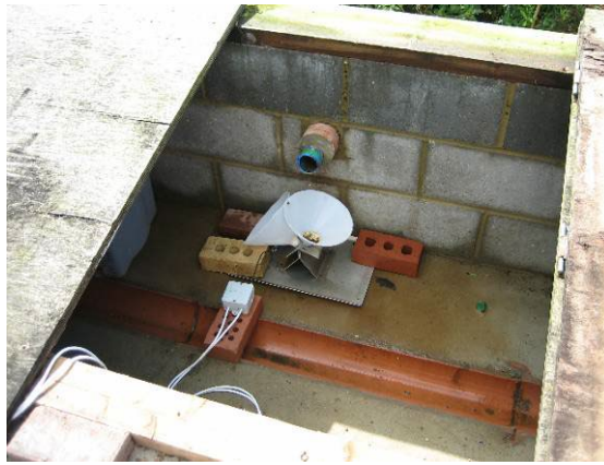
Figure 13. Tipping buckets used to monitor run-off from beds. Tips of the buckets were automatically recorded and the total number of tips read daily. This was then converted to litres of water.
