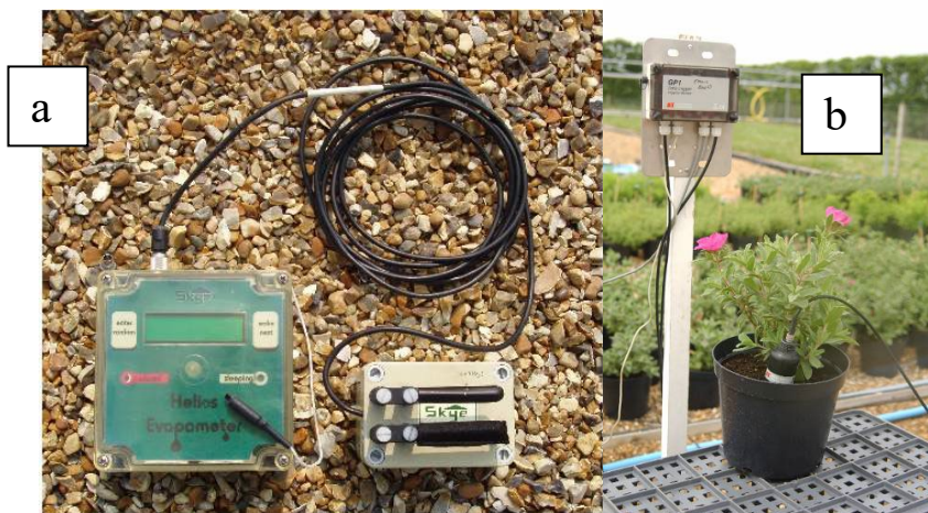
Figure 3. Different technology for scheduling irrigation on the EMWC: Evaposensor and EvapoMeter (Skye Ltd.) (a) and soil moisture in-pot sensor with GP1 logger (Delta-T Devices Ltd.) (b)
