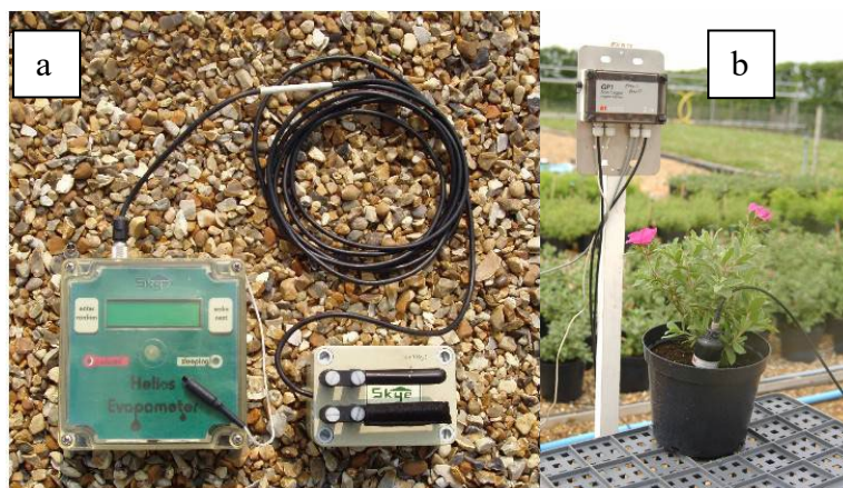
Figure 4. Different technology for scheduling irrigation on the EMWC: Evaposensor and EvapoMeter (Skye Instruments Ltd.) (a) and soil moisture sensor and GP1 (Delta T Devices Ltd.) (b).
